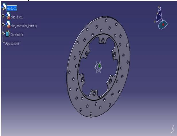
Fig 2.Design Model of Disk Brake
