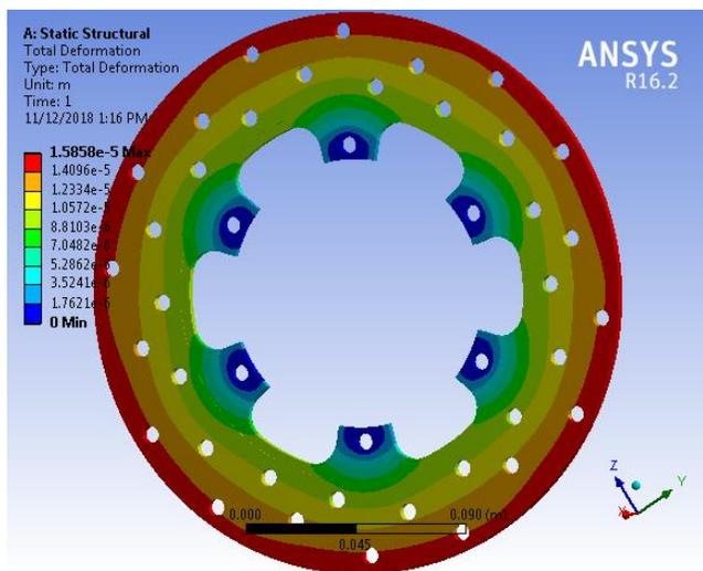
Fig7. Deformation of Disk Without air hole
