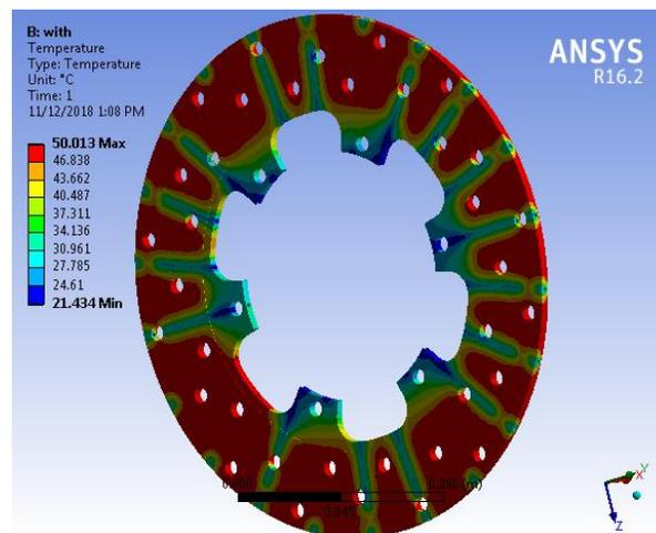
Fig 10. Temperature distribution of with air hole of disk brake
