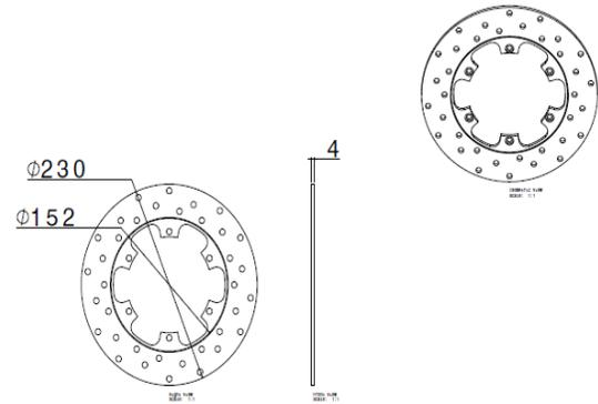
Fig 3.Detailing of Disk Brake
